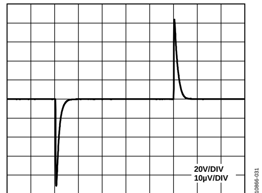
Figure 31. Operational Amplifier Load Transient Response (100 \mu A Load Change)
